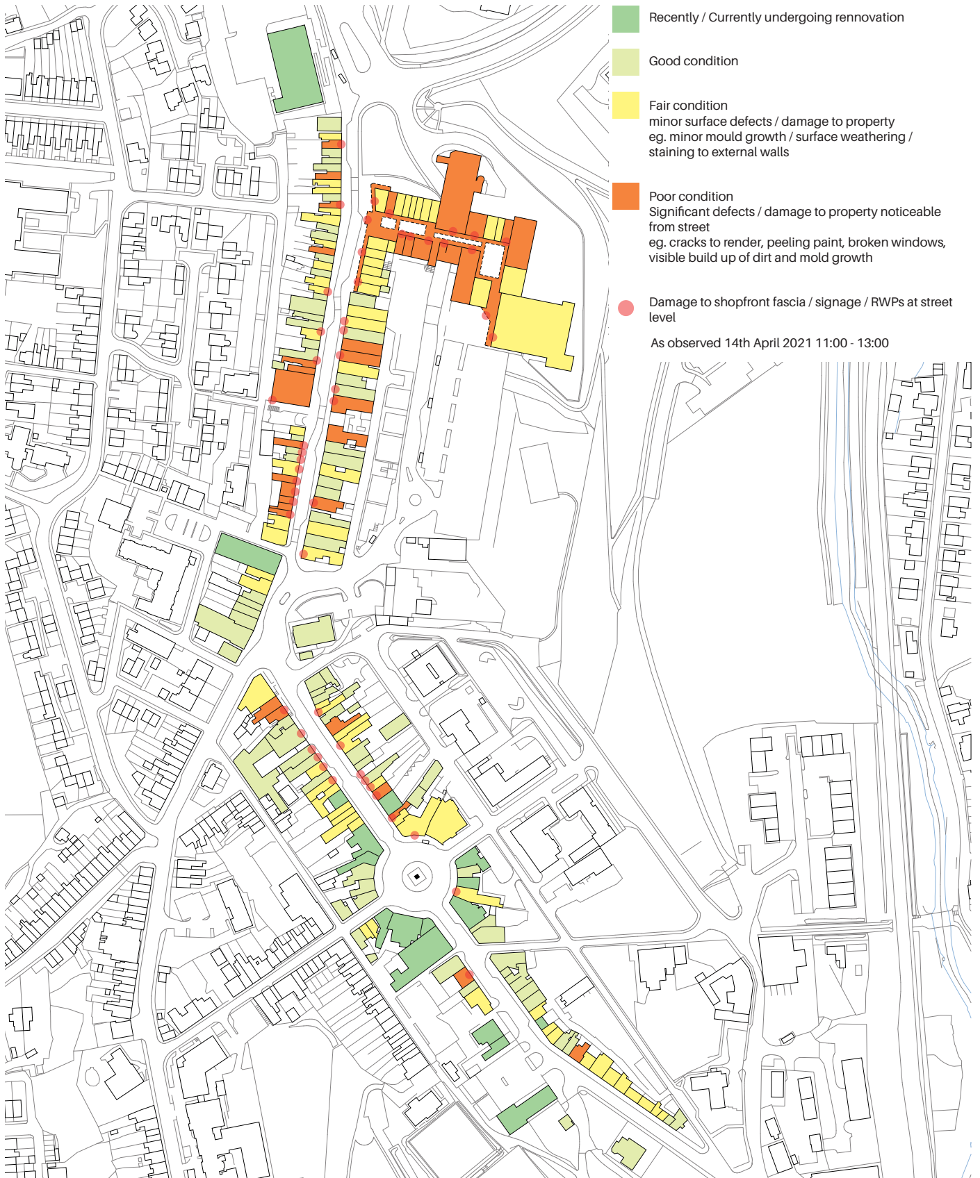
FIG. 6 BUILDING CONDITION SURVEY
